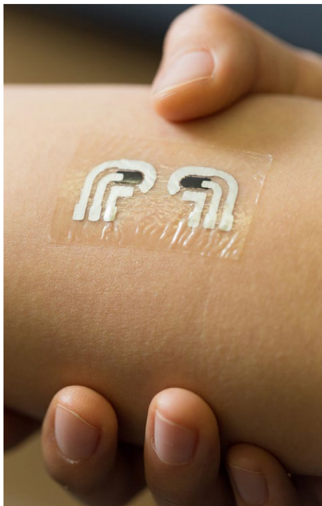
Figure 15: Printed electronics tattoo with diagnostic tools on board.
