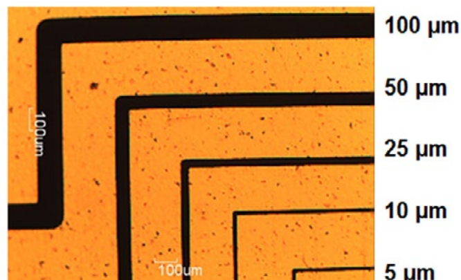
Figure 2: Fine lines on polyimide flex material.
